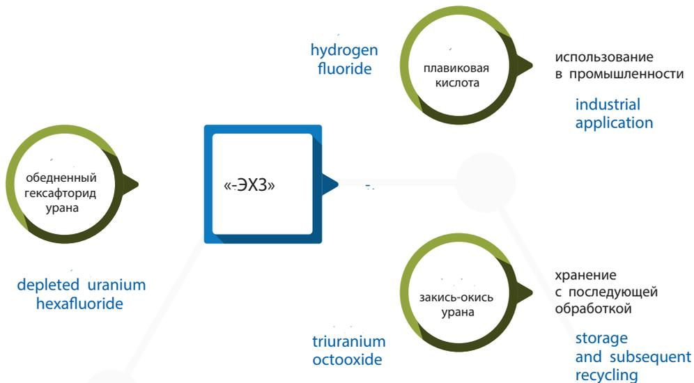
W-ECP fully recovers fluorine from  $\text{DUF}_6$ . It was designed to reduce the amount of stored  $\text{DUF}_6$  in the facility by recycling  $\text{DUF}_6$  into  $\text{U}_3\text{O}_8$  and hydrogen fluoride.
